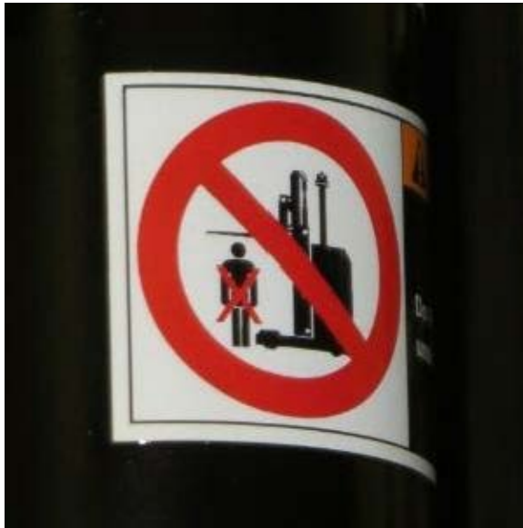
Sticker on the LGV indicating that working underneath elevated forks was prohibited.
