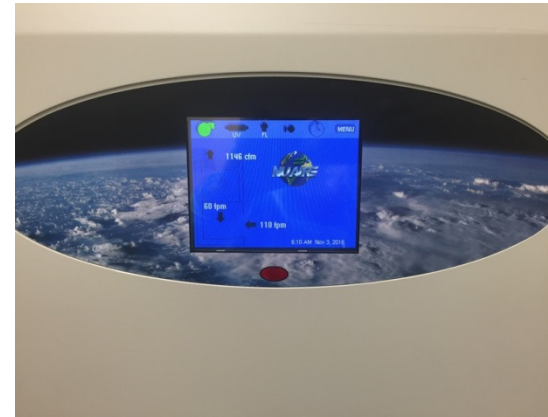
Integrated airflow monitoring devices on BSC
