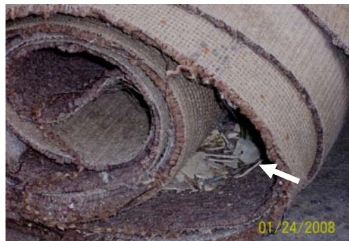
VAT debris rolled up in carpeting
