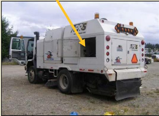
Photo below shows **better** back-up alarm location; external and facing the backing zone.
