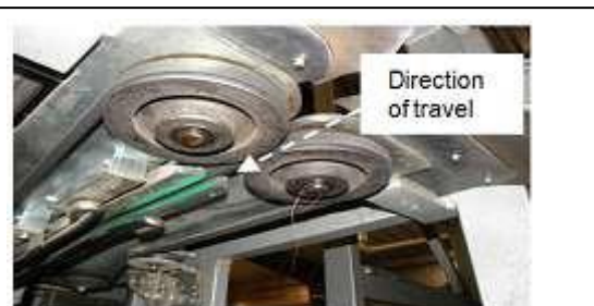
Photo 2. The metal clamp (underside shown without an attached bag) has moved from the extended position shown in Photo 1 to a fully retracted position on the other side of the rollers.
