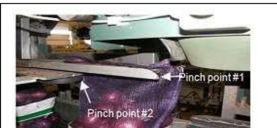
Photo 1. Unguarded and dangerous: metal clamp arms extend and come together (pinch point #1) to grab the bag and pull it through rollers (pinch point #2) and on towards the stitcher.
