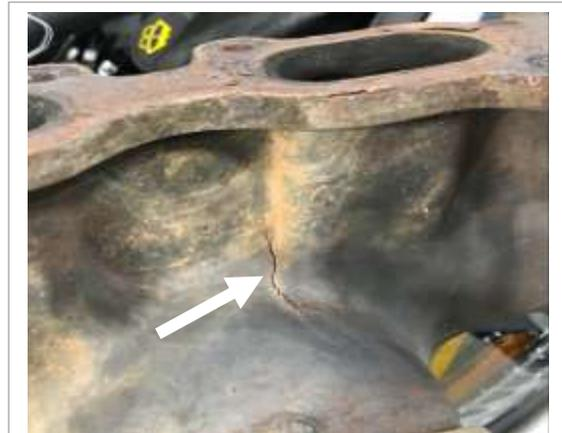
**Warning!** Cracks in vehicle exhaust manifolds (see arrow) can allow harmful carbon monoxide (CO) gas to enter the engine compartment and flow into the cab through the ventilation system. Photo: L&I
