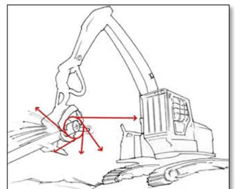
Chain shot is thrown in multiple directions along the plane of the saw bar. It can also ricochet off objects.
