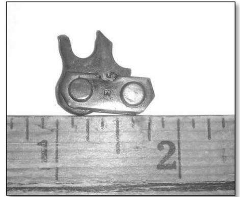
**A small size but a deadly threat:** chain shot from harvester or processor heads and stroker-log merchandisers or delimiters can maintain lethal velocity after **penetrating ½-inch thick polycarbonate windshields.**
