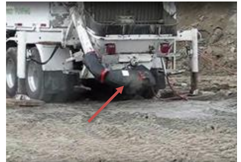
A transition shield like the one shown here is one safety measure that can keep workers safe from blowouts.
