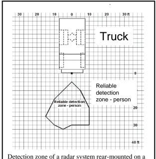
Detection zone of a radar system rear-mounted on a truck to detect a pedestrian. Source: Ruff<sup>4</sup>.
