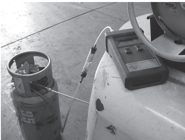
In-house forklift emissions testing.
