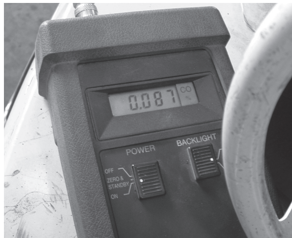
In-house forklift emissions testing.
