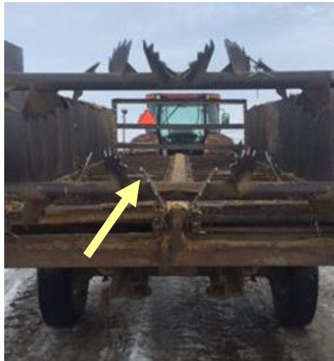
Photo of straw spreader bars. Arrow indicates where worker's clothing was entangled in rotating beater bar.
