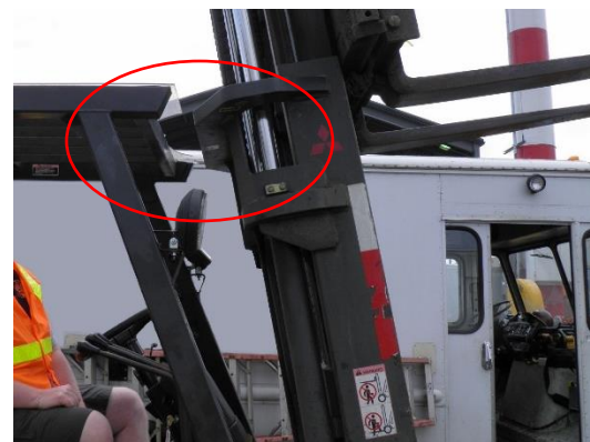
Forklift mast in the full tilted back position. The red circle indicates the area where the victim's torso was crushed between the cross member of the overhead guard and the mast.
