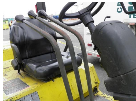
Forklift control levers used to adjust the forks and mast. The middle lever is the mast tilt lever.
