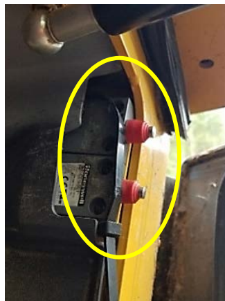
Buttons released as designed when cab door is open.
