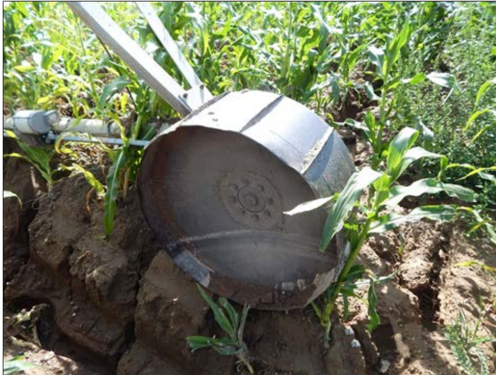
Photo 3. The 38-inch diameter steel wheel at the base irrigation system's tower that ran over and crushed the operator.
