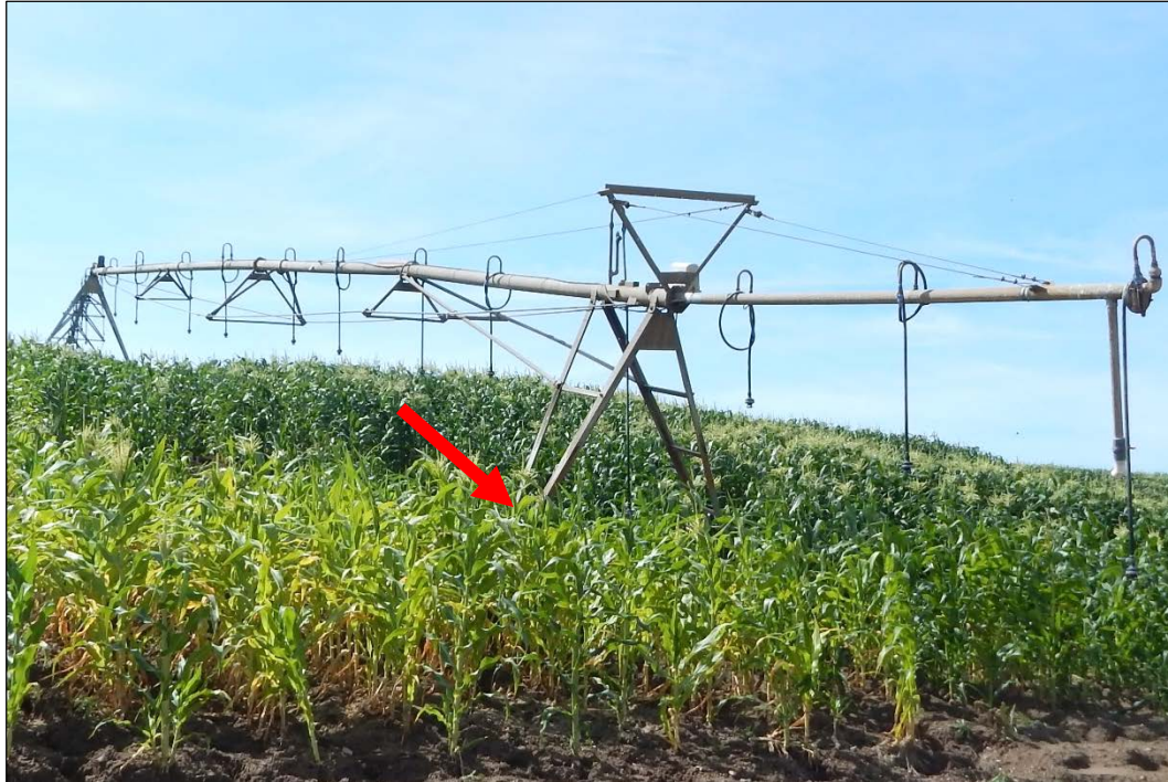
Photo 1. Incident scene with self-propelled center pivot irrigation system. A wheel (indicated by the arrow) at the base of the system's tower ran over and crushed the operator.
