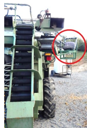
Chair (indicated by circle) from which the laborer fell.
