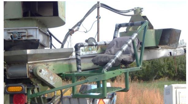
Chair installed by employer from which the laborer fell.
