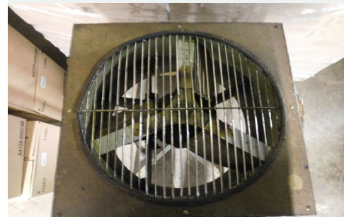
Photo 2: The bud trimming machine the worker was using when her gloved finger went into the fan blade and was amputated.
