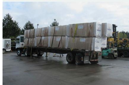
**Incident 2:** The trailer and load in the photo are similar to the trailer and load in the second incident where the truck driver fell from the top of the load.
