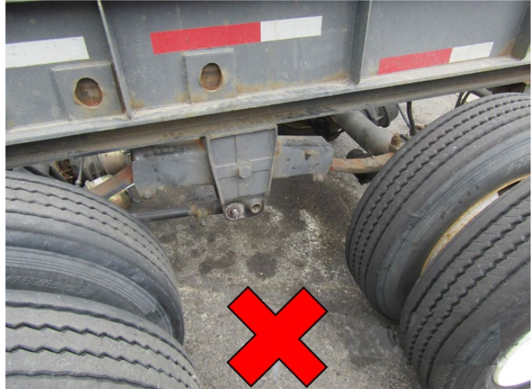
Red X shows where mechanic was trapped and crushed by the rollaway chassis' wheels.
