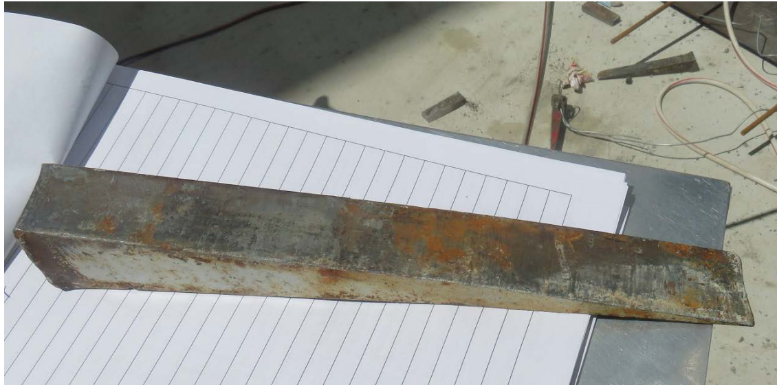
Photo 4. Steel wedge that struck the apprentice ironworker in his upper back near his left shoulder.
