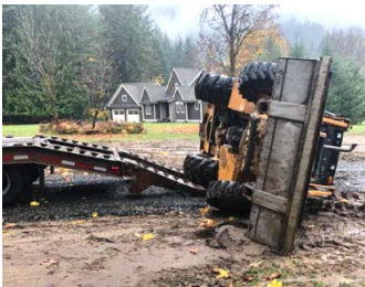
Overturned backhoe and trailer. The driver was not wearing the seatbelt and was crushed under the ROPS.
