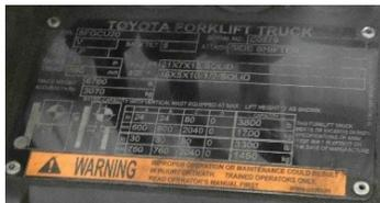
Yellow warning label on incident forklift's instrument panel. The label provides a warning that improper forklift operation or maintenance could result in injury or death.
