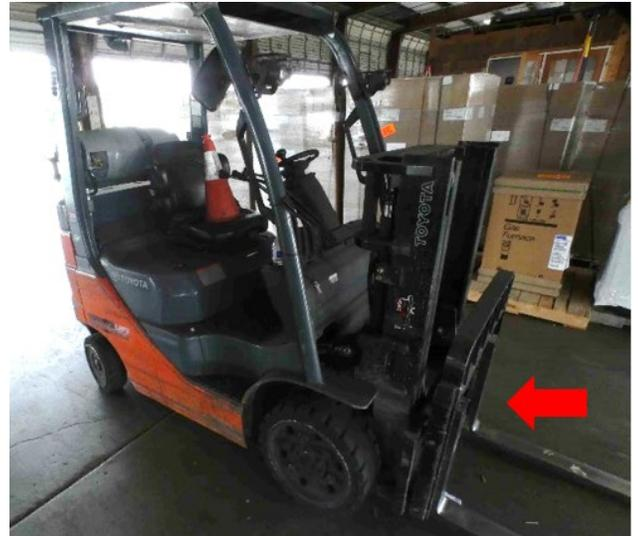
Arrow shows lowered mast on incident forklift. The operator leaned forward in the cab, reached his arm through the mast's crossmembers, and inadvertently engaged the control lever that dropped the mast on his arm, crushing it.
