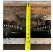
Close up of 11-inch unguarded gap above chain and sprocket drive where worker reached in and mangled his hand.
