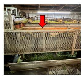
Hop harvester machine in which worker mangled his hand trying to remove debris. Arrow shows gap above horizontal steel mesh guard and chain and sprocket drive where worker reached in. Note machine's lack of hazard warning and LOTO signage.
