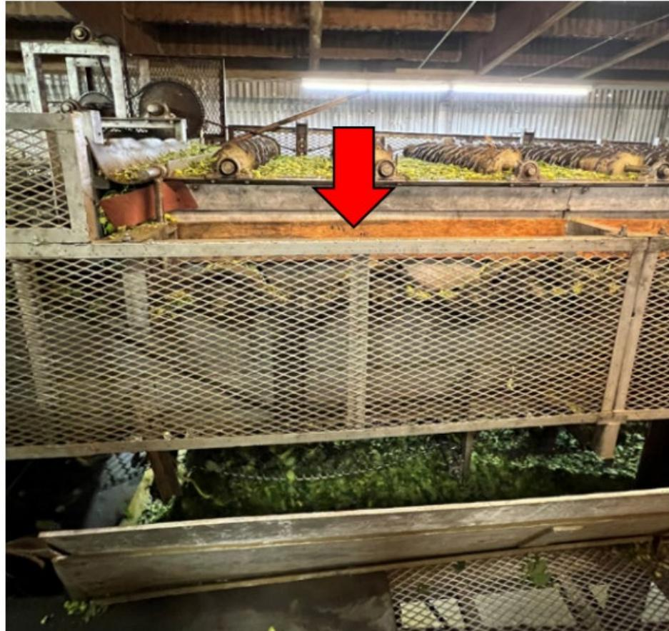
**Photo 1.** Hop harvester machine in which worker mangled his hand trying to remove debris. Arrow shows gap above horizontal steel mesh guard and chain and sprocket drive where worker reached in.
