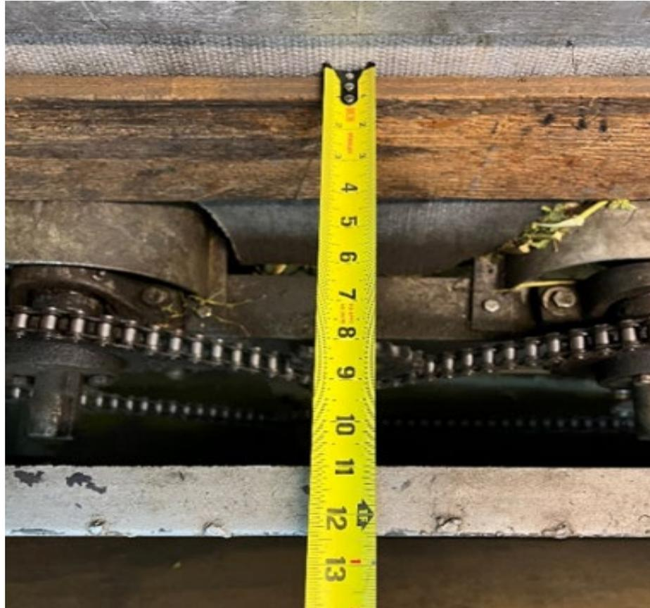
**Photo 2.** Close up of 11-inch unguarded gap above chain and sprocket drive where worker reached in and mangled his hand. Torn pieces of the worker's glove were found in the chain after the incident.
