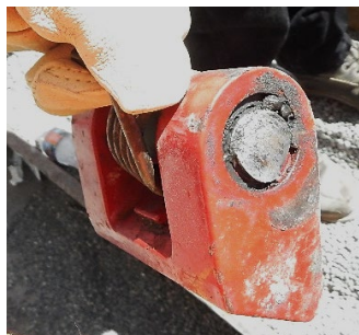
The safety knuckle that detached from the quick coupler.
