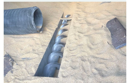
Incident 2: The injured worker was shoveling grain around the tube on the left. The auger was covered with steel plates during the incident.
