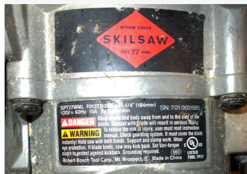
The label on the saw clearly states to hold the saw with both hands. It also warns if the blade binds, the saw may kick back.
