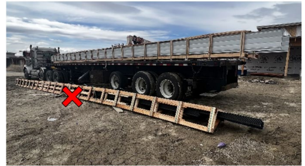
Location (x) where truck driver was crushed by crate that was pushed off the trailer by a forklift on the other side.
