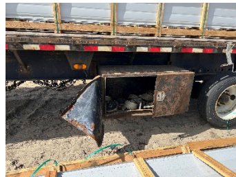
Damage to trailer's underbody toolbox caused by crate that crushed driver.
