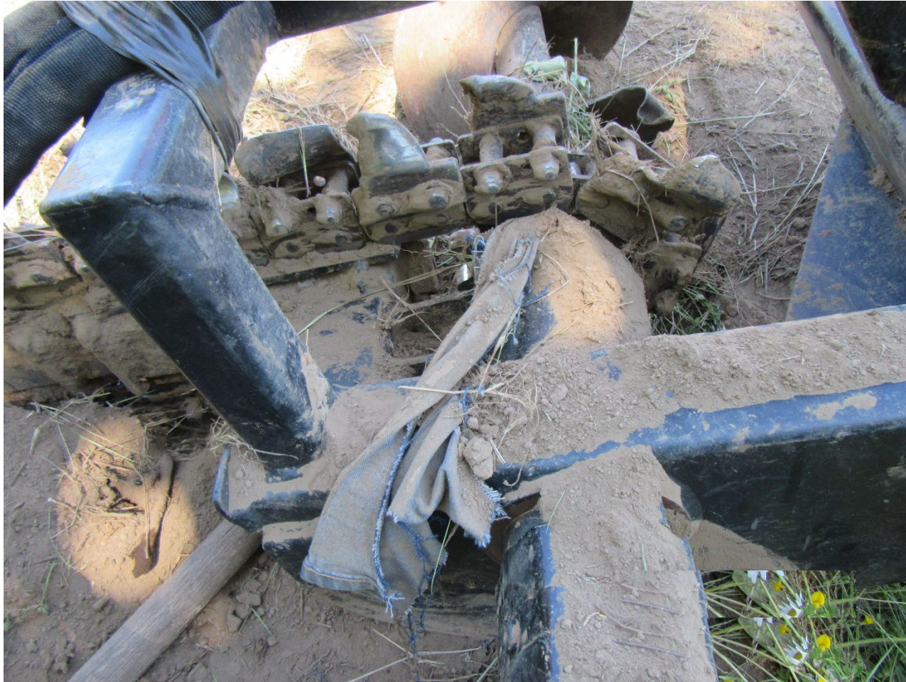
Photo 4. Close up of trencher roller chain and digging teeth.
