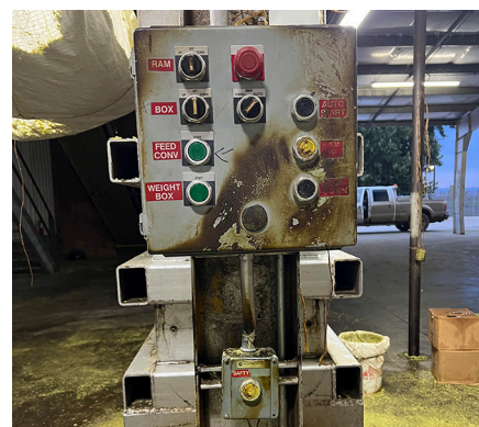
Control panel located on one side of the hop baler.
