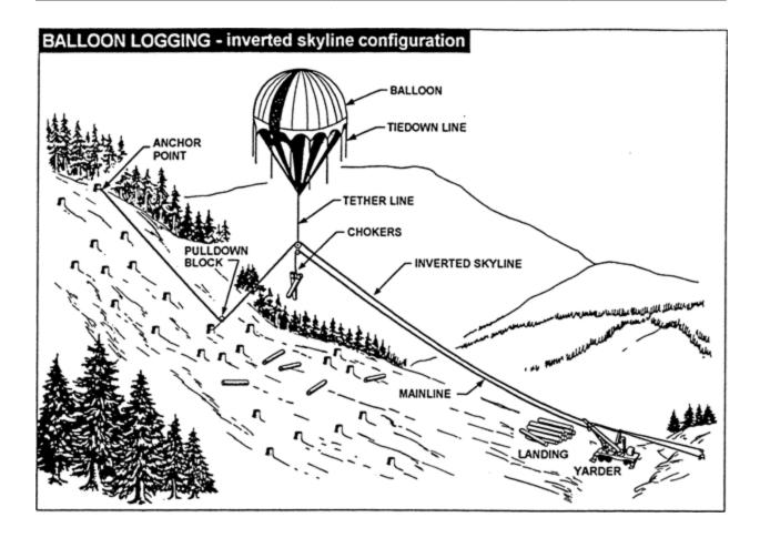
**Figure 57: Balloon Logging - Inverted Skyline Configuration**
