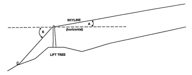
Figure 16: Positioning Guylines in Back of Tree
