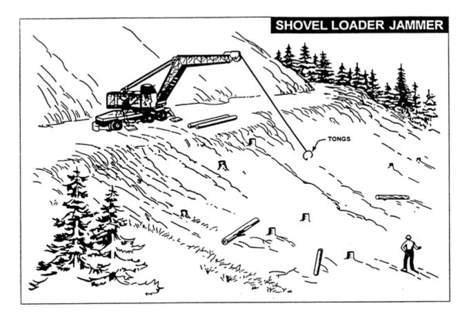
**Figure 43: Shovel Load Jammer**
