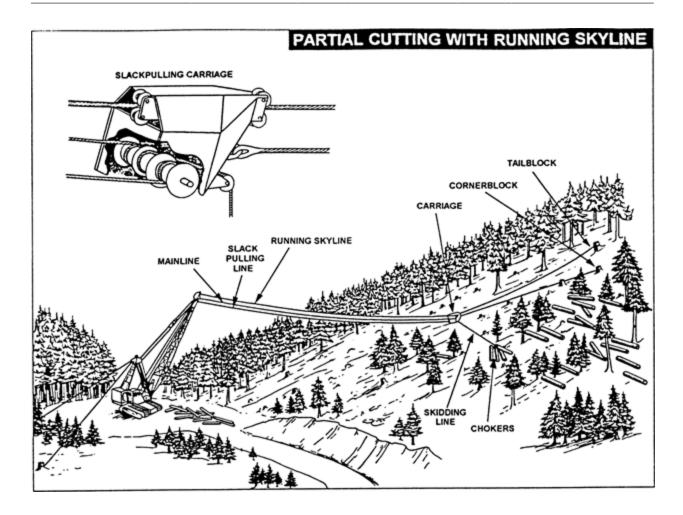
Figure 53: Partial Cutting with Running Skyline
