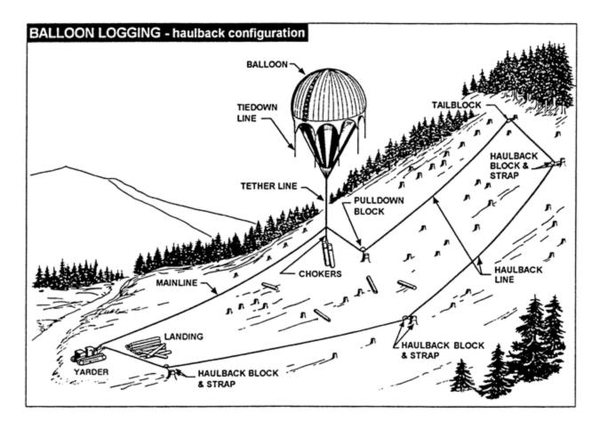
Figure 58: Balloon Logging - Haulback Configuration
