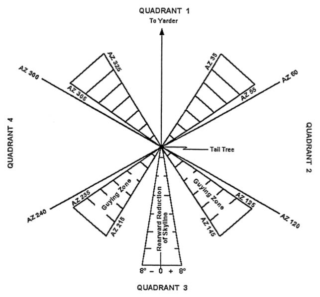
Figure 23: Skyline Positioning Limits Tail/Lift Tree
