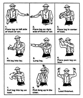
Figure 42: Standard Signals for Loading Logs
