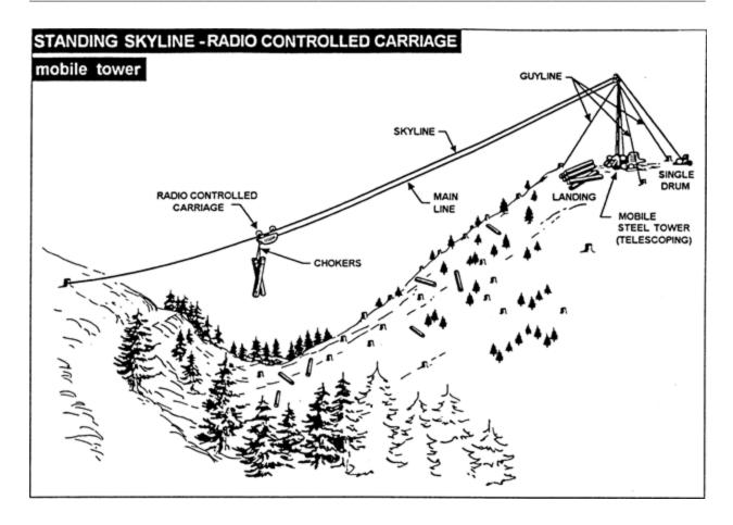
Figure 51: Standing Skyline - Radio Controlled Carriage - Mobile Tower
