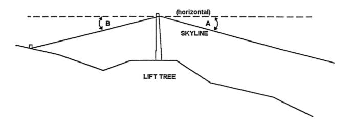
Figure 17: Positioning Guylines in Front of Tree
