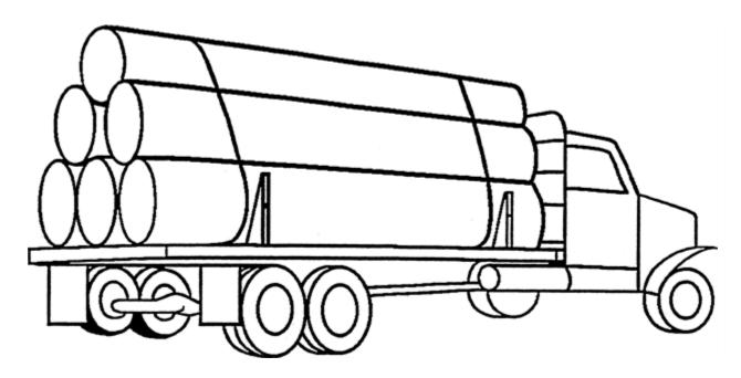
Figure 29: Five or Six Log Load All Logs 17 feet or less Seven or More Log Load All Logs 17 Feet or Less
