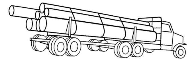
**Figure 32: Proper Support for Logs**
