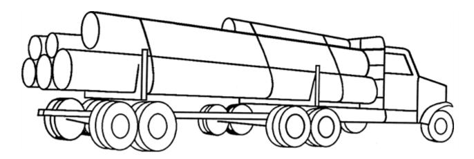
Figure 34: A Wrapper must be near each bunk
