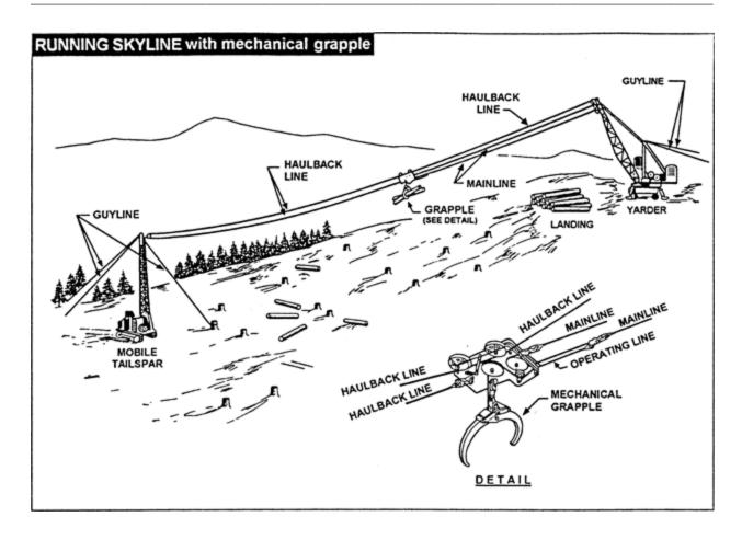
Figure 55: Running Skyline with Mechanical Grapple
