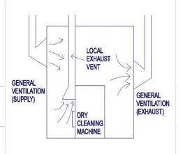
For better ventilation: the direction of air flow should move from a clean area (customer counter) to one that's less clean (machine area) where vapor is captured and vented outdoors by local exhaust and a wall-mounted exhaust fan.
